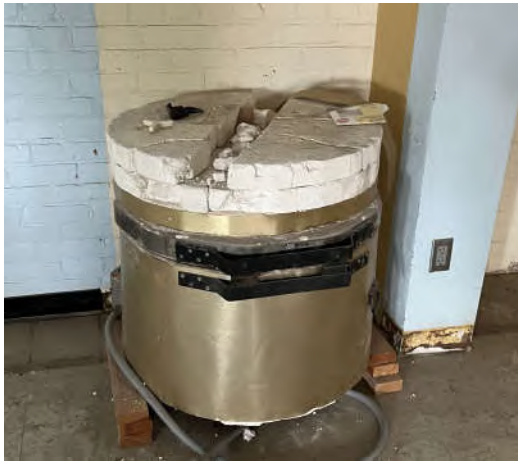
Photo 7: Kiln identified for removal as part of the asbestos abatement scope.
